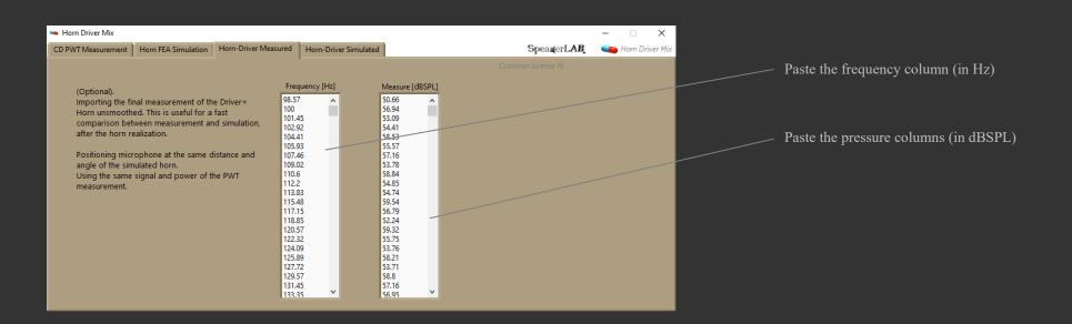
Prediction vs Measurement/Target
