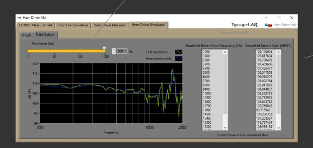
Copy Hz and dBSPL columns into your spreadsheet or measurement system
