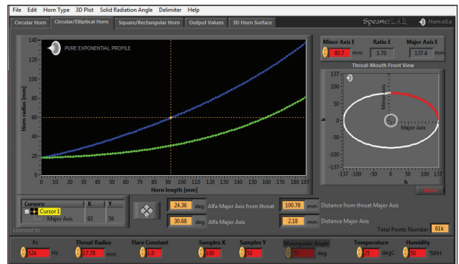
Figure 18: Elliptical mouth horn's arrangement. MR = 1.7
