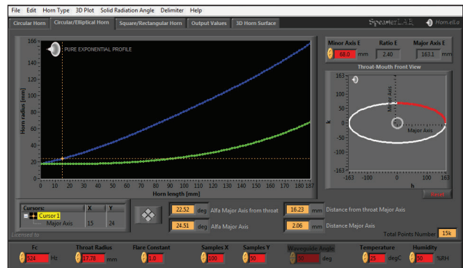
Figure 19: Elliptical mouth horns arrangement. MR = 2.4
